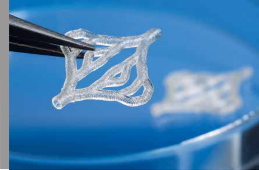
Branched microtubes as well as complete microfluidic systems for biomedical analysis technology.
