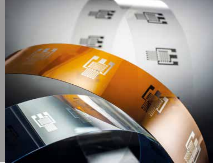
Printed and laser functionalized strain gauge sensors on polymer foils.
