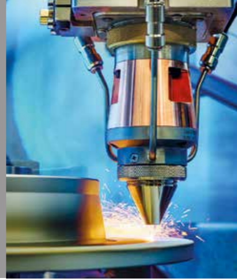
Coating a brake disc with the EHLA process
